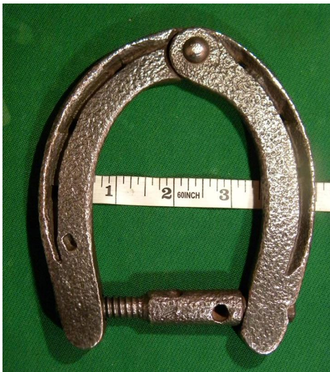
Figure 12. A version of shoe designed to 'force' the heels open. Circa 1800's. With kind permission of Mr D.Bradbury MBE FWCF, Clay Cross farriery museum.
